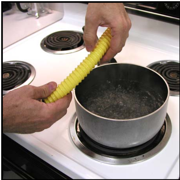
Photo #3 Let hose cool for a 5-10 seconds and then using your fingers reshape the hose.
