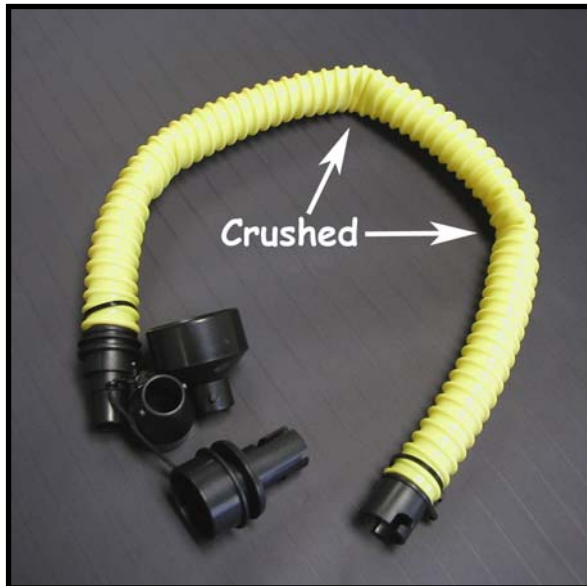
Photo #1 Damaged Hose
