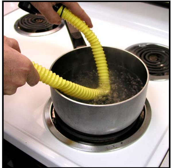
Photo #2 Dip Hose into boiling water for 10 seconds .
