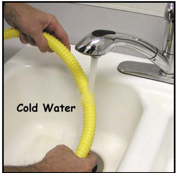
Photo #4 Place hose under cold water for 10-20 seconds or until the hose has cooled.
